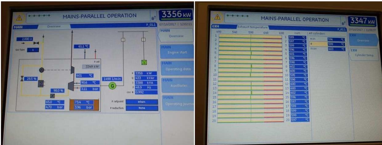
Fig. 2. Control panel exhibiting operating data of gas engines.
